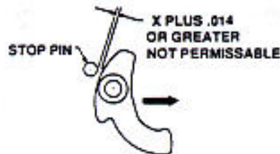
FIGURE 5. FLYWEIGHT TO AXLE WEAR CHECK
