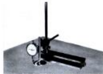
Figure 4. Method of Checking Valve Edge Thickness with Dial Indicator
